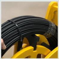
DO NOT remove the ties or plastic packaging until the coil is attached to the caddy and ready to use.
