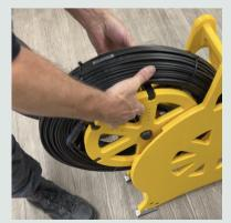
Reinsert the loaded spool into the caddy frame.
