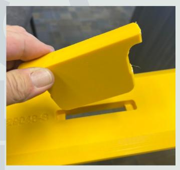
Insert Yellow Fins from the top side and press into place until flush with the surface.
