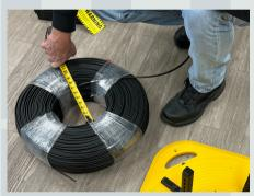
Determine the Internal Diameter by measuring the coil.
