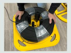
Lower cable onto coil stops.
