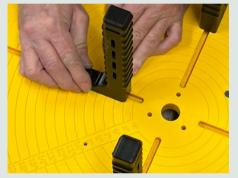
Adjust the 4 coil stops by loosening the knobs, sliding the stops inwards or outwards and adjusting them to the proper ID by aligning the arrow on each stop to the corresponding circular diameter guide.
