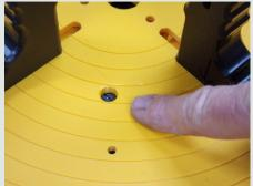
The turntable spinning rate can be adjusted to add more drag by adjusting the large screw.
