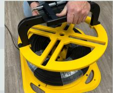
Reattach the MFT/MST tray by aligning the tray over the stops. The tray rides onto the cable and adds pressure to the coil as the coil is unwound.
