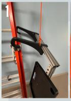
**Attach handline to** platform using pre-approved handlining procedures.
