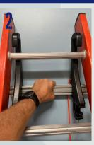
Once handlined up, hang device onto rung at desired location.
