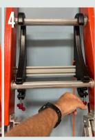
Secure in place with Red adjusting clamps
