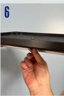
Secure Splicing Machine to platform using captive knob provided.
