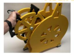
Remove spool from caddy frame by sliding the spool assembly from the frame.
