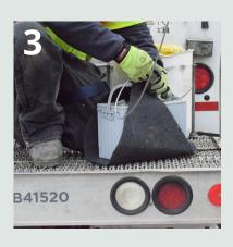
Attach Battery sling to the carabiner clip on the end of the winch line and place battery on the shelf to raise.
