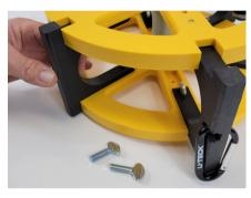
Slide the spacers to the desired spool diameter by removing the thumb screws and reinserting in the desired position.
