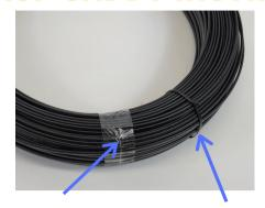
DO NOT remove the ties or plastic packaging until the coil is attached to the caddy and ready to use!
