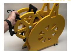
Remove spool from caddy frame by sliding the spool assembly from the frame.
